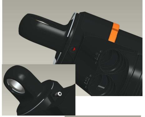
Place the shock tube in clamping block part no 90100040 (See picture). Use tool part no 90100005S to tighten the contra nut. Torque: 75 Nm
