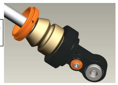
Put tool part no 90100039 over the pistonrod tap and mount the holder part no 46000050S1/2/3
